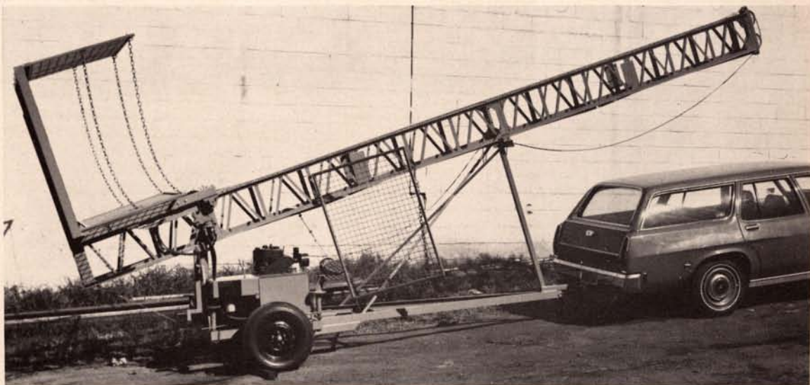
The Pannell Plant Mark 10 Drive-up Drive-down Builders' Hoist takes to the road on the completely demountable trailer.
